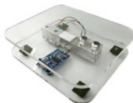
Fig. 6.8 Arduino development board and weight sensor
